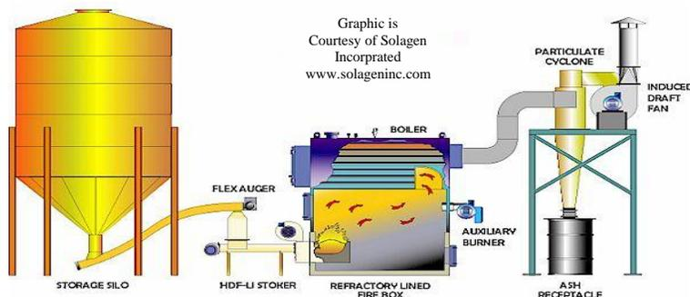
**Boiler Plant Technology:** The boiler plant is a biomass based system with a firebox, automatic feed stoker with under-fire air. The system can be configured to produce hot water, low or high pressure steam and can be couple with a steam let down turbine for additional electric generation benefits. Boiler's range from 100 hp to 1,500 hp.
